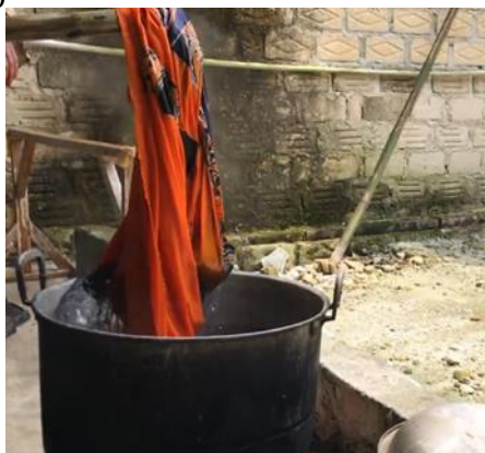
Figure 2. The process of ngelorod, process of boiling and rinsing the batik fabric to remove the wax
